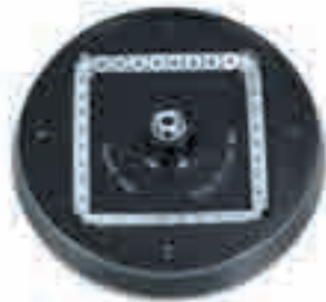
PCR Rotor - CODE 1052 32 x 0.2 ml Tubes 15000 RPM / 21206 X g
